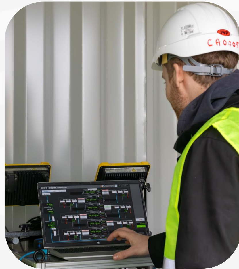
The air management system for automatic and manual inflation/deflation of each panel
