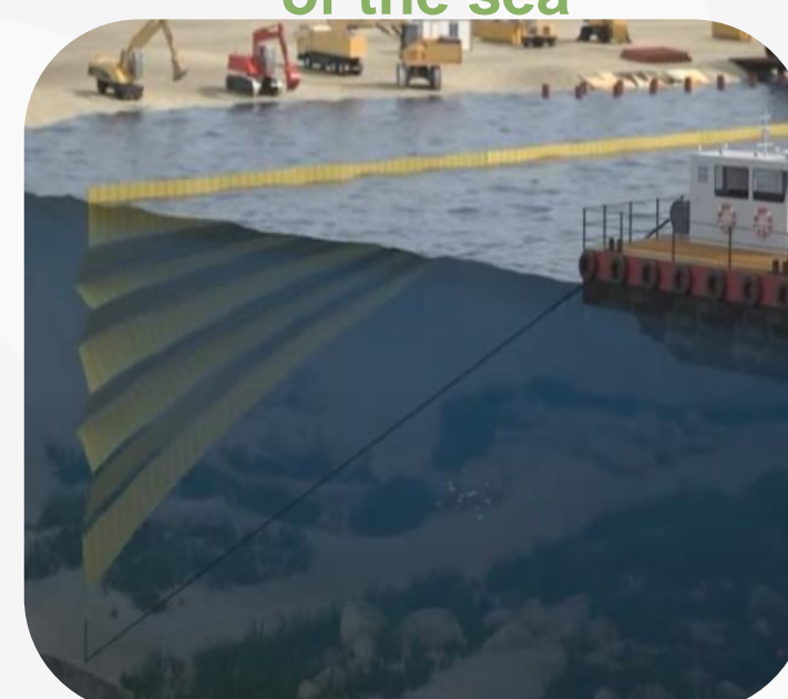
Mooring of the SSQ in the chain at the bottom of the sea
